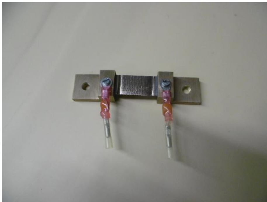
Fig 3: Shunt, new installation
