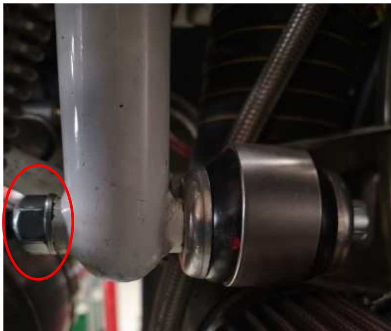
Engine mount assembly with SI full metal M10 nut
