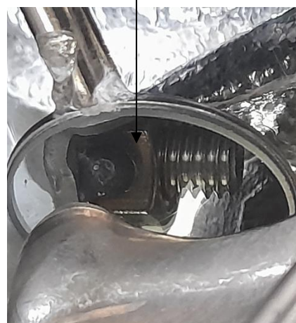
Fixed nut on the turbo charger bracket
