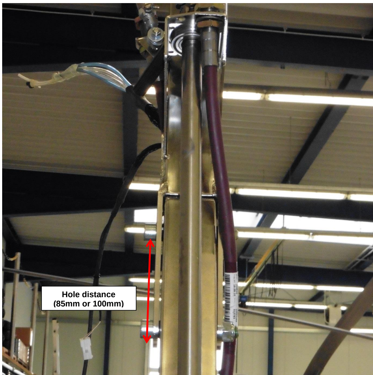
Fig 3: Calidus upper to lower mast connection hole distance
