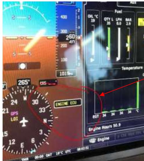
Should an engine error occur, the exact error information can be called up during the flight.
