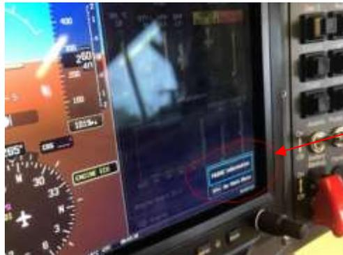
The FADAC Information will now open. The error shown below was provoked by disconnecting the Ambient Pressure sensor plug.
