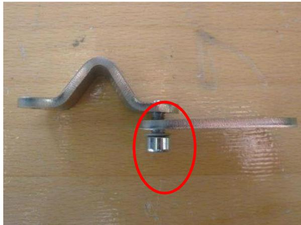
Fig.1 Joined PPC clamp and PPC V-clamp
