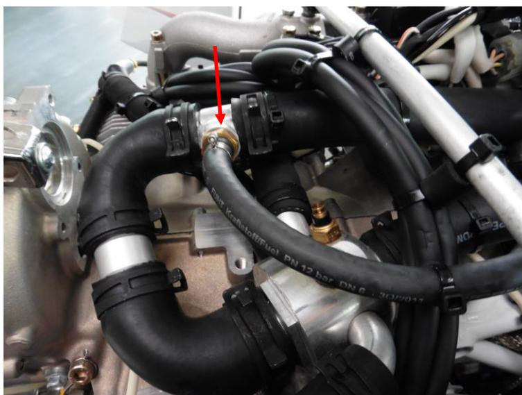
Fig.2: Connection between expansion tank and highest point at T-connection
