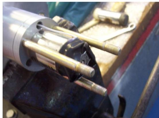
9. Using a plastic mallet tap the end of the leadscrew through the flange until the motor and planetary gearbox are released. **Caution – do not drop the gears! NOTE! The small gear on the end of the motor is a slide fit!**
