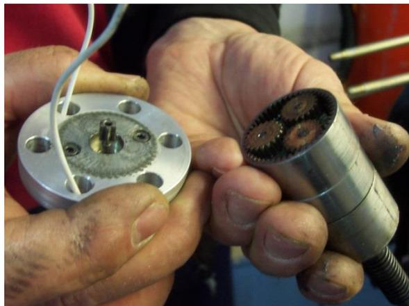
10. There are three layers of gears. During dismantling and cleaning be sure to keep the layers together as a set.
