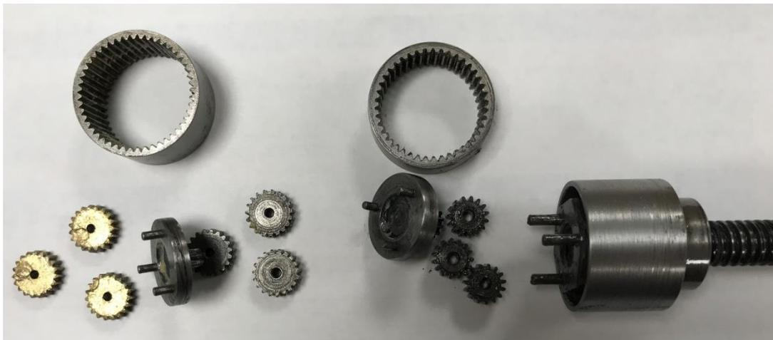
11. Using suitable solvent (e.g., Amberklene LO30) or brake cleaner thoroughly clean all grease from the gearbox assembly and motor mounting plate.
