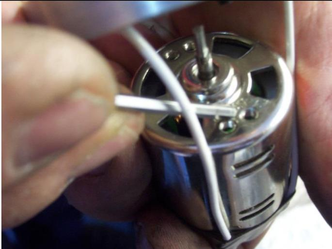
14. Visually inspect the gearbox components for burrs (remove as necessary) then re-pack the gearbox assembly with Molykote BR2 Plus (or equivalent) and re-lubricate the leadscrew assembly with Molykote and internal thrust bearings with Ballistol oil (Part number 88-00-00-S-31816)
