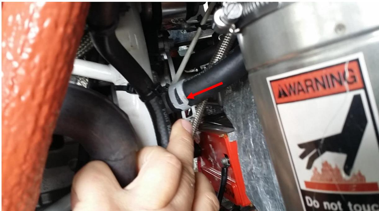
Fig. 2 clamp at engine end of water hose
