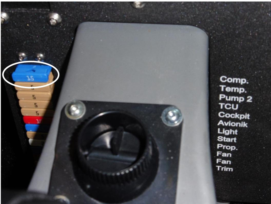
Fig. 2: 15A Fuse Compressor
