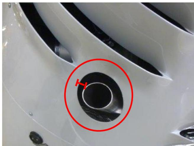
Fig.7: Position of the muffler tube
